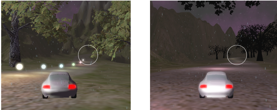
(a) Due to the limit of ten light sources, the lights closest to the car were used when calculating the lighting. The circle shows the intended position of the distant lights which are not contributing. (b) Deferred lighting allowed more light sources to affect objects in the scene and the distant light sources are now contributing.
